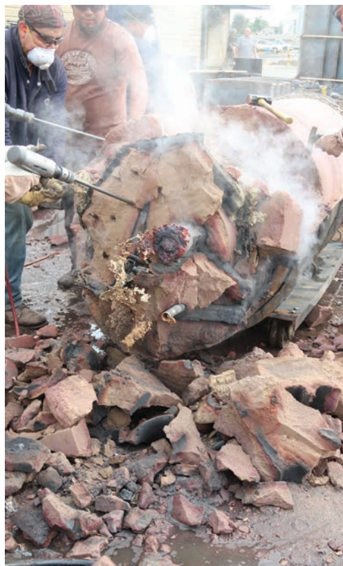
▲ Resin bonded sand is broken away from the tree, exposing the gating system which transports molten metal in and around the tree trunk, and allows gasses to escape from the casting process.
