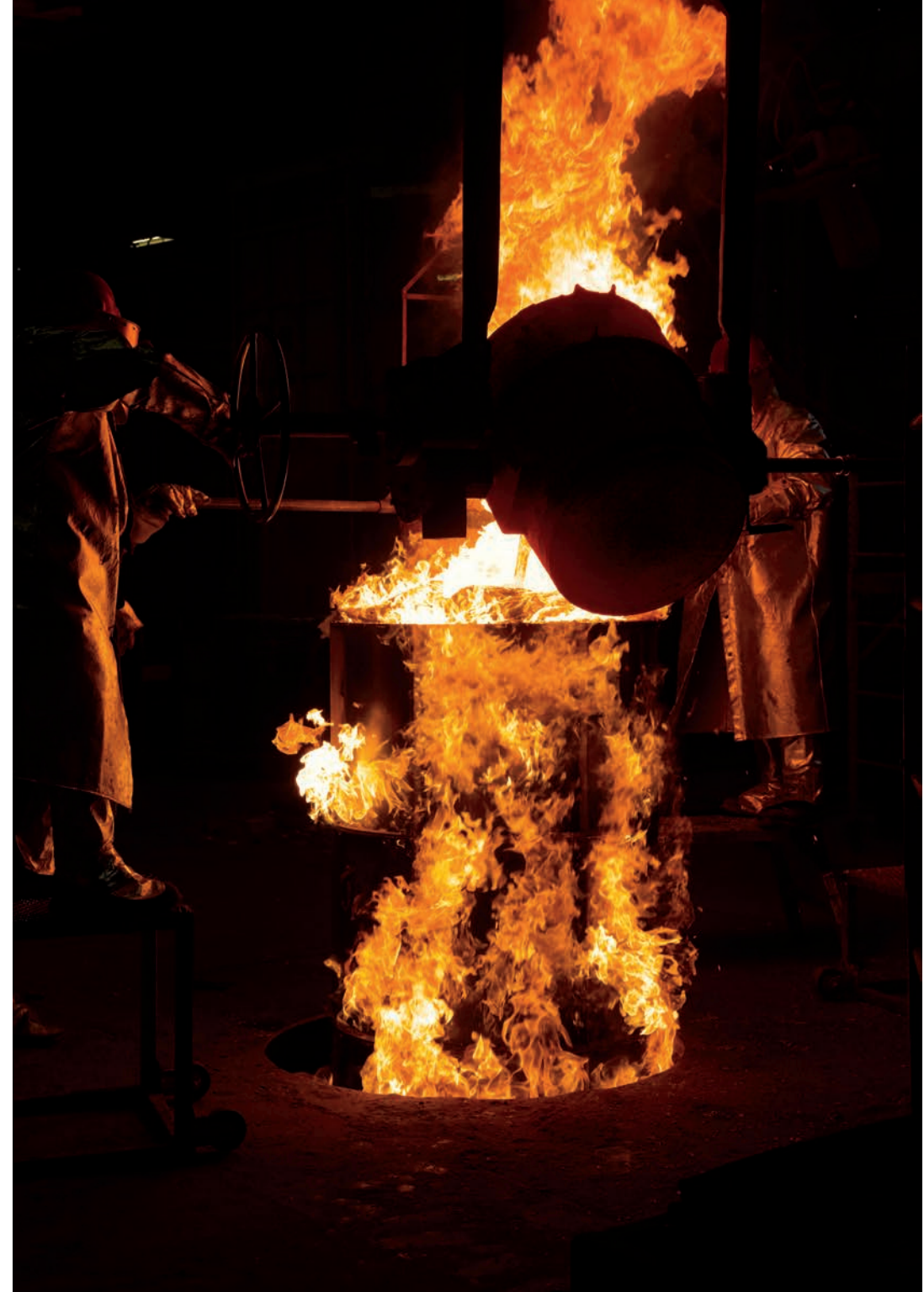
◀ Molten copper and brass are poured into the vacancies between the sand mold and the tree, incinerating the foam and replacing it with metal. A deep pit has been excavated in the floor of the casting room to hold the mold.
