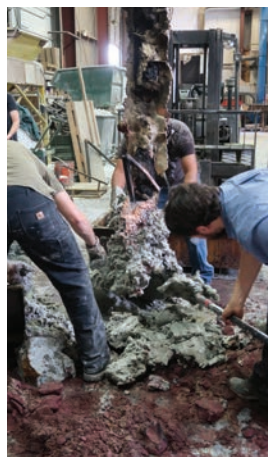
▲ Molten copper and brass exiting the end of the tree trunk is captured in a vat of bentonite clay and water. The clay slurry creates cavities for the metals to chill without forming an alloy, leaving a marbled combination of the two metals.
