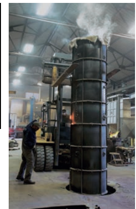
◀ The steel flask containing the mold is removed from the casting pit. From the heat of the molten metals, the tree is still smoldering inside the sand mold.
